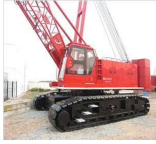
Radius guard is missing on this crane
