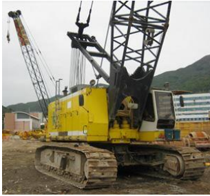
Radius guard is missing
