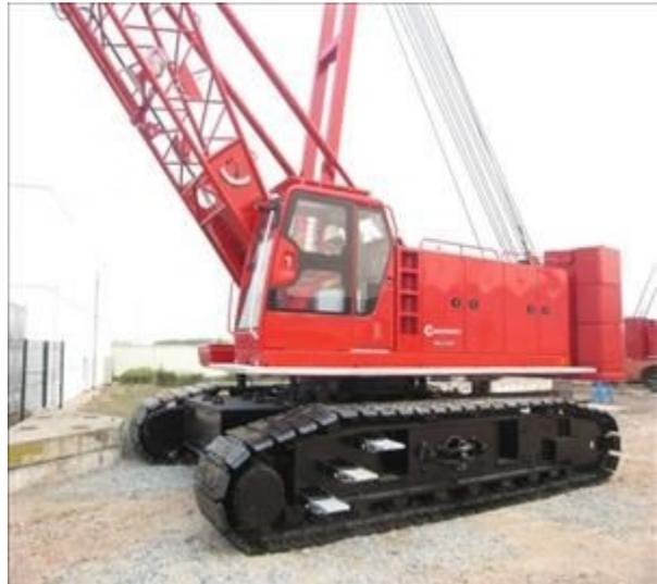
Radius guard is missing on this crane
