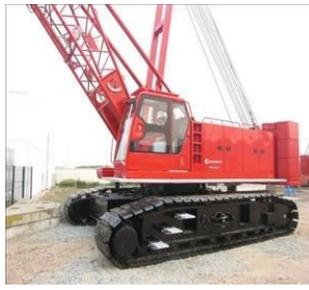
Radius guard is missing on this crane
