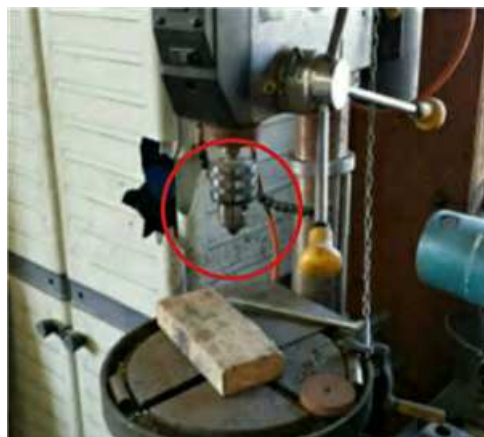
Chuck guard needed on drill press
