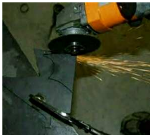
Guard missing on grinder
