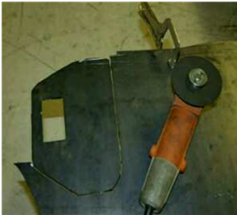
Guard missing on grinder
