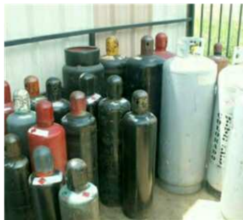
Cylinders not secured to prevent tipping
