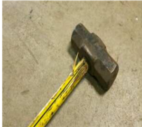
Damaged shaft on hammer
