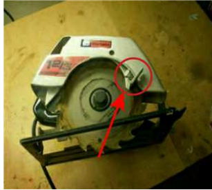
Self-adjusting guard is bypassed
