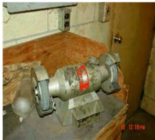
Grinder is not mounted to bench top
