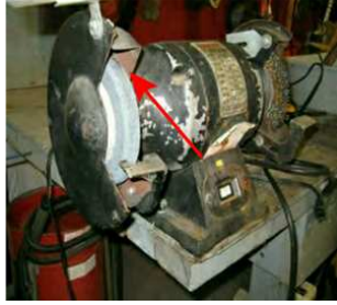
Tongue guard missing
