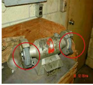
Guards missing on bench grinder
