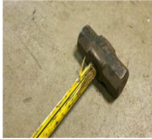
Damaged shaft on hammer
