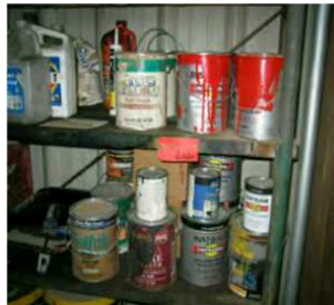
Flammable not stored properly
