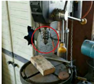
Chuck guard needed on drill press
