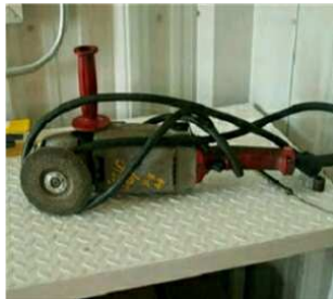
Guard missing on angle grinder
