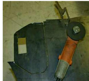
Guard missing on grinder
