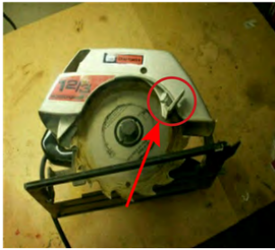
Self-adjusting guard is bypassed
