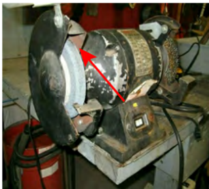
Tongue guard missing
