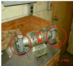
Guards missing on bench grinder
