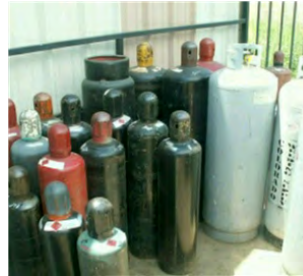
Cylinders not secured to prevent tipping
