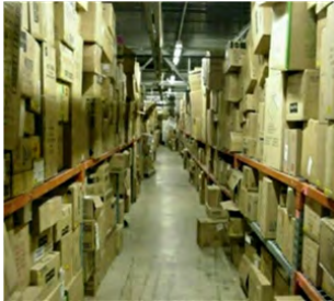
Product stored in warehouse needs to be banded or use shrink wrap when staking on top shelf.
