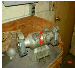
Grinder is not mounted to bench top
