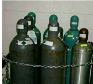
Proper Cylinder storage
