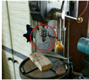
Chuck guard needed on drill press
