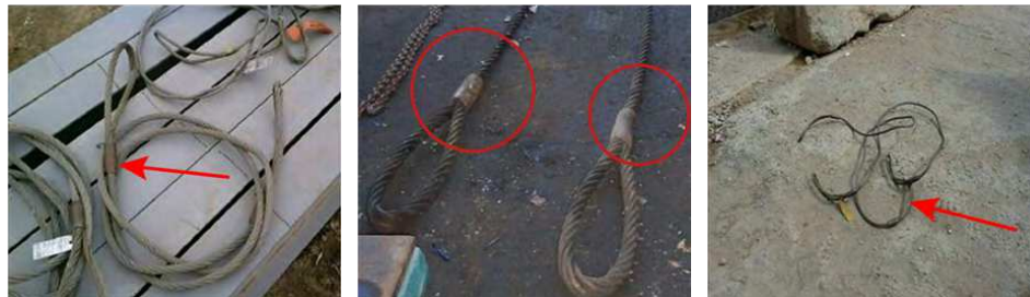
Specification tag missing
